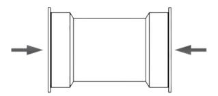
**3** - Apply grease to the bottom bracket axle and bottom bracket bearings. Insert a 0.5mm plastic washer against the chainring if in chainline 49, otherwise against the flat spacer of chainline 52 then place the bottom bracket axle inside the bottom bracket.
