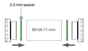
2 - Apply grease to the bottom bracket axle and bottom bracket bearings. Insert a 0.5mm plastic washer against the chainring if in chainline 49, otherwise against the flat spacer of chainline 52 then place the bottom bracket axle inside the bottom bracket.
