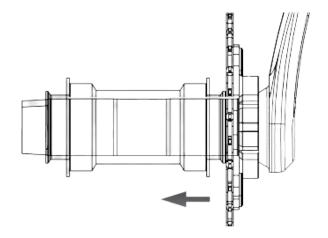
**3** - Insert the number of washers (0.5/1mm) needed to perfectly adjust the tightness of the bottom bracket. Insert the wave washer and tighten the bottom bracket screw until the wave washer becomes flat and the bottom bracket turns freely without any resistance or play.
