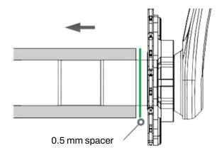
4 - Insert the wave washer and tighten the bottom bracket screw until the wave washer becomes flat and the bottom bracket turns freely without any resistance or play.
