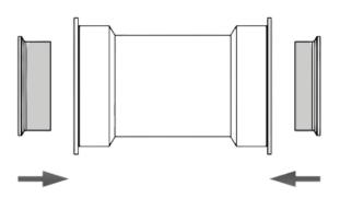
**2** - Apply grease to the bottom bracket axle and bottom bracket bearings. Insert the bottom bracket axle into the bottom bracket.
