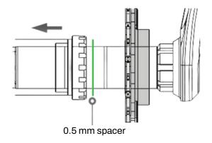
**3** - Insert the number of washers (0.5/1mm) needed to adjust the tightness of the bottom bracket. Place the wave washer and tighten the bottom bracket screw until the wave washer becomes flat and the bottom bracket turns freely without any resistance or play.
